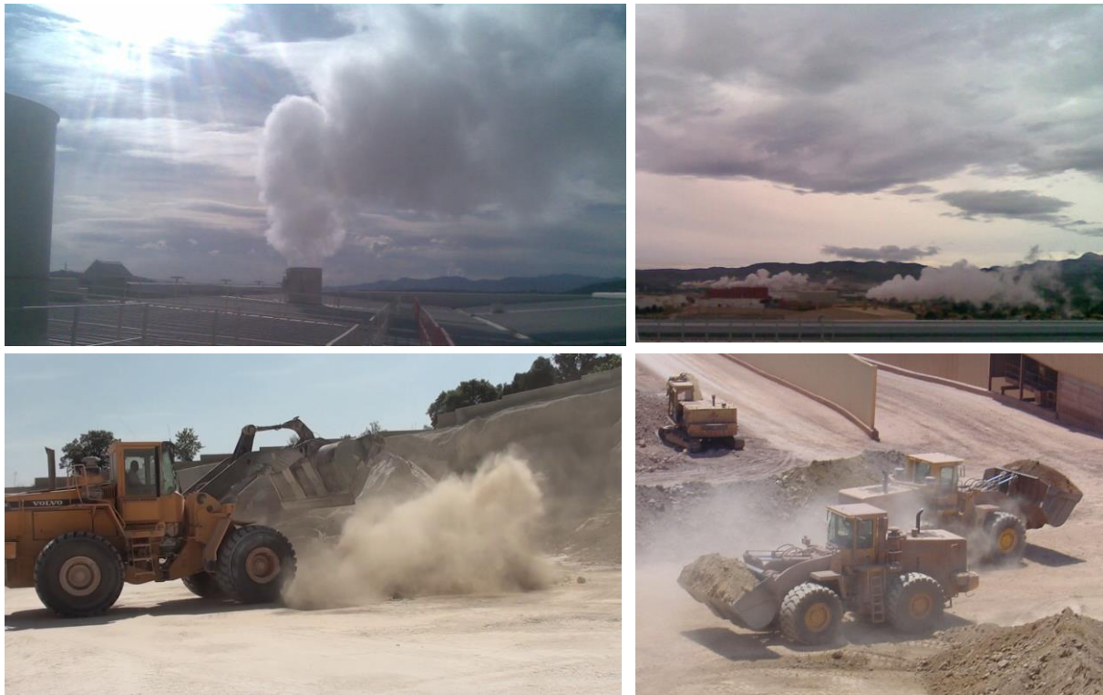
Figure 7. Channelled (top) and fugitive (bottom) PM emissions from industrial sites. Source: ITC-AICE
