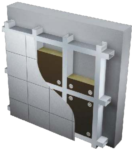
Metal façade insulation system
